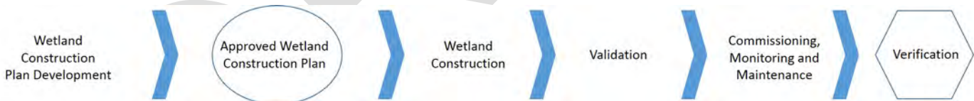
Figure 1. Wetland construction process steps.
